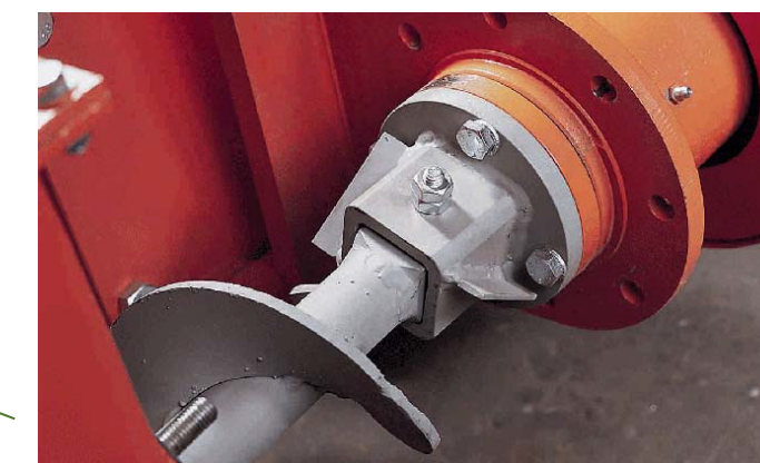
Screw pivots around a universal joint on one end thereby allowing the screw to avoid oversized pieces inside the pipe housing
